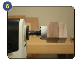
Attach the workpiece to your wasteblock. Typically for pendants and small, flat objects, double stick tape is the preferred mounting method. For large stock glue is recommended.
