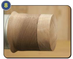
With your blank turned, remove the tailstock and slightly dome the face of your pendant. Sand your workpiece to the finished grit.
