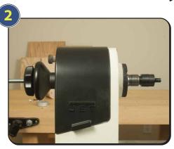
Install the black washer and thread the knob on to the thread of the drawbar and secure. NOTE: The draw bar is intentionally made extra long to fit most any lathe. You may cut the bar shorter if desired.
