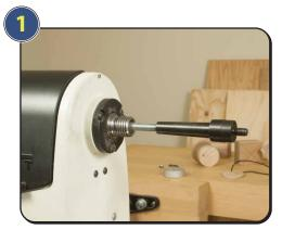
Insert the MT-2 mount into and through the headstock spindle on your lathe.
